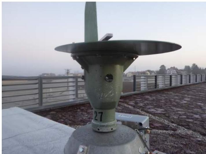
Two standard Hirst-traps were iced and the heated one was not. Obviously, the weather conditions on this February morning ( $T^\circ$  between  $-1$  and  $-2^\circ$  C and  $rH > 90\%$ ) were not particularly favourable for pollen emission and airborne dispersion. However, there is a clear risk of reduced monitoring efficiency in certain conditions and should be considered for studies in cold and humid areas.
