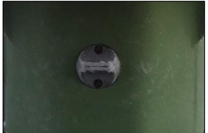
The first test was conducted on the roof of MeteoSwiss building in Payerne. The pictures above were taken early in the morning of February 15th 2017, and show the icing of the inlet of the trap.
